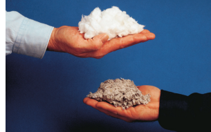
Fiber glass insulation (top) is a more fire-resistant choice than cellulose (bottom).
