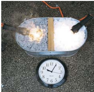
AFTER 5 MINUTES: Smoldering combustion had begun in the cellulose side. There was no effect on the InsulSafe.
