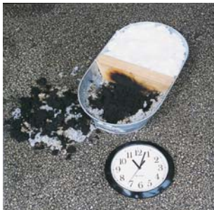
AFTER 60 MINUTES: Combustion had consumed most of the cellulose, causing significant damage to the wood. Again, no effect on the InsulSafe.
