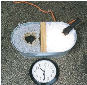
AFTER 30 MINUTES: Combustion continued to spread in the cellulose. The light, inserted back into InsulSafe, still had no effect.
