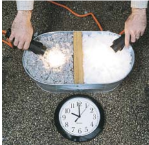
A heat source using a 60 watt bulb placed on cellulose insulation and InsulSafe® fiber glass blowing insulation.
